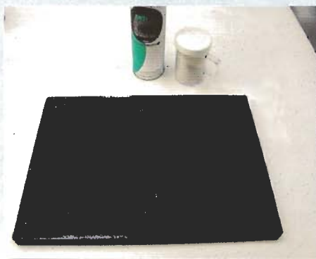
3. Seal particulate with a second coat of AntiSkid Spray
