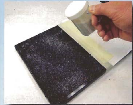
2. Sprinkle with particulate
