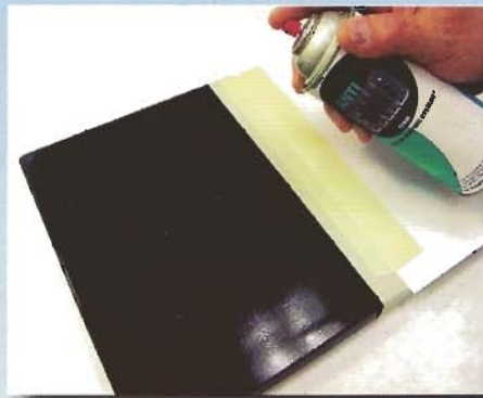
1. Apply AntiSkid Spray to part
